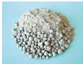
Artificial zeolite used in Hitachi air purifier filters
